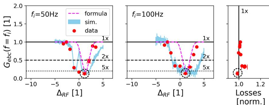
(a) Measured (data), simulated (sim.) and semi-analytical (formula) ripple magnitudes  $G_{\text{abc}}$  as a function of RF-frequency offset  $\Delta_{\text{RF}}$ . Beam loss data (right subplot) have been vertically aligned with their corresponding  $G_{\text{abc}}(f_i = 100 \text{ Hz})$ .
