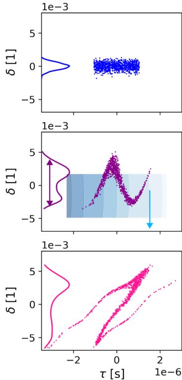
Figure 3: Simulation of phase displacement blow-up in the PS at  $h = 1$ . The momentum distribution is shown before (top), during (centre) and after (bottom) the manipulation, with the blue arrow and colour map (centre) showing the direction and location of the zero-area ‘empty bucket’, respectively.
