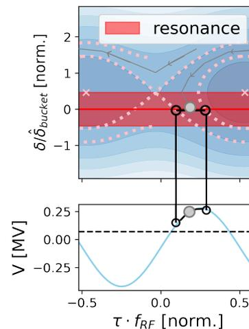
Figure 1: Illustration of the empty bucket channelling technique. Particles cross the resonance separatrix (top) while sampling the RF wave crest (bottom). The time of arrival  $\tau$  and the relative momentum offset  $\delta$  have been normalised by the RF frequency  $f_{RF}$  and the bucket height  $\hat{\delta}_{\text{bucket}}$ , respectively.
