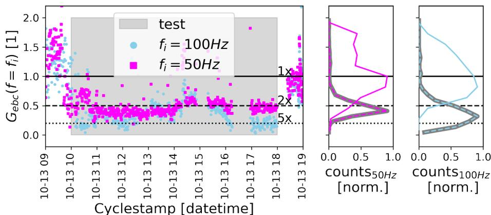
(b) Cycle-by-cycle measurement of ripple magnitude  $G_{\text{abc}}$  with cycle timestamp ‘month-day hour’ in x-axis (left), and cumulative histograms (right). Plots show channelling at fixed optimised RF settings (grey filling) and RF off (no filling).
