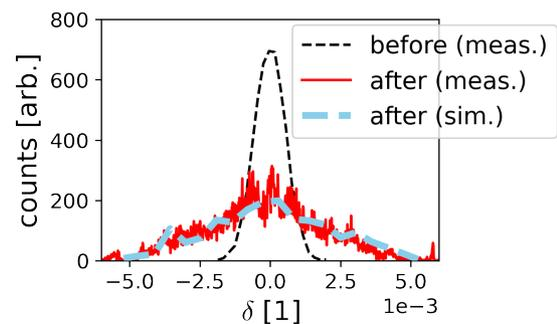
Figure 5: Beam-momentum distribution before and after phase-displacement blow-up.
