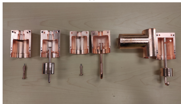
Figure 1: Mechanical design (a) and 3D-printed plastic and copper-coated prototypes (b) of the Probe, Hook, and DQW HOM couplers (from left to right).
