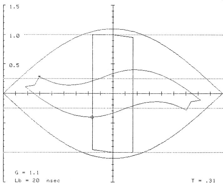
At middle of bunch : V = .336Tip (point No.13): V = .285 shown by: \* Lowest (point No. 5): V = -.403 shown by: 0
