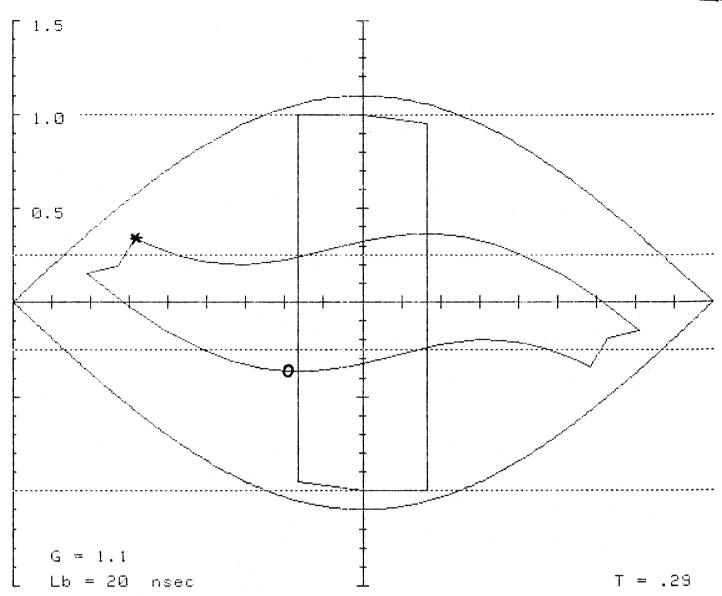
At middle of bunch : V = 1.324Tip (point No.13): V = 1.343 shown by:  $\bigstar$ Lowest (point No. 5): V = -1.364 shown by:  $\bullet$
