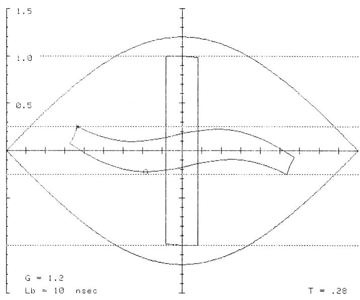
At middle of bunch : V = .177Tip (point No.13): V = .252 shown by: \* Lowest (point No. 5): V = -.223 shown by: 0
