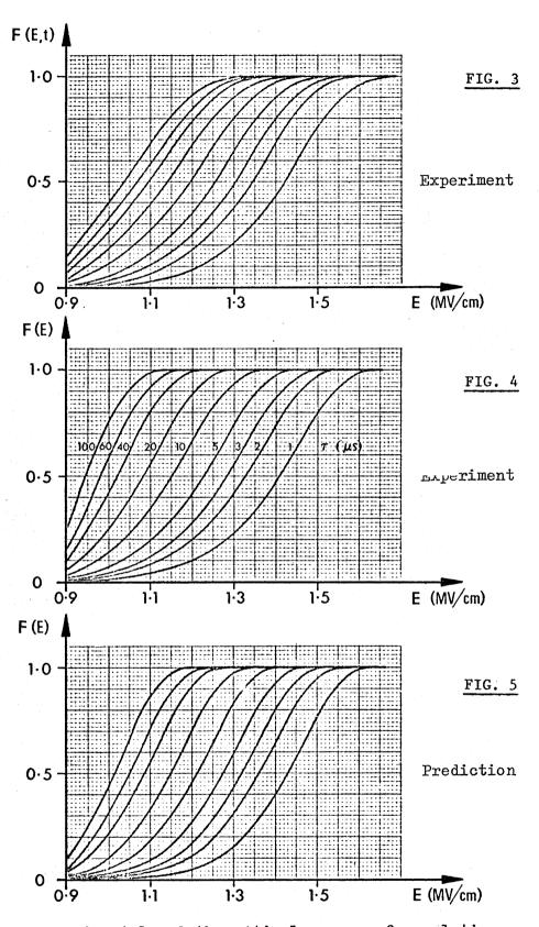
Experimental and theoretical curves of cumulative probability vs. Stress for several pulse widths at a gap of 34  $\mu$ m.
