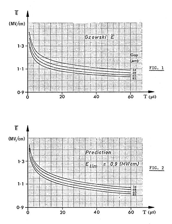
Experimental and theoretical curves of Mean Breakdown strength vs. Pulse width for several sphereelectrode spacings.
