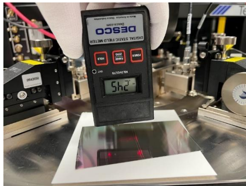
Figure 1. Electrostatic charge measurement on sensor surface during initial reception tests. Displayed value is in units of kVolts.
