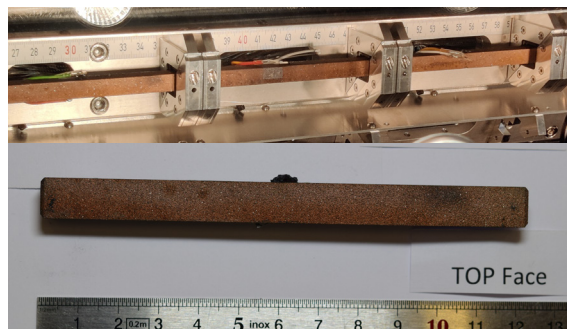
Figure 5: CuCD. Top: in-tunnel visual inspection of the target line. Bottom: HD image of the most loaded sample.
