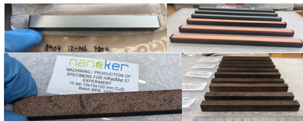
Figure 2: Top left: Mo-coated MoGr. Top right: Mo and Cu-coated graphite. Bottom: CuCD.
