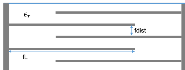
Figure 4: Sketch of the silver fingers applied to \text{Al}_2\text{O}_3 .
