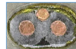
Twinax cross-section (Molex)
