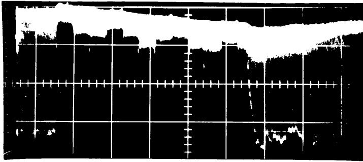
Fig. 2 : Radial beam displacement in ss 83. Quad. 73 shunted with 2 \Omega Fk 95 attenuated 11% ( 5 \mu\text{s}/\text{div} )
