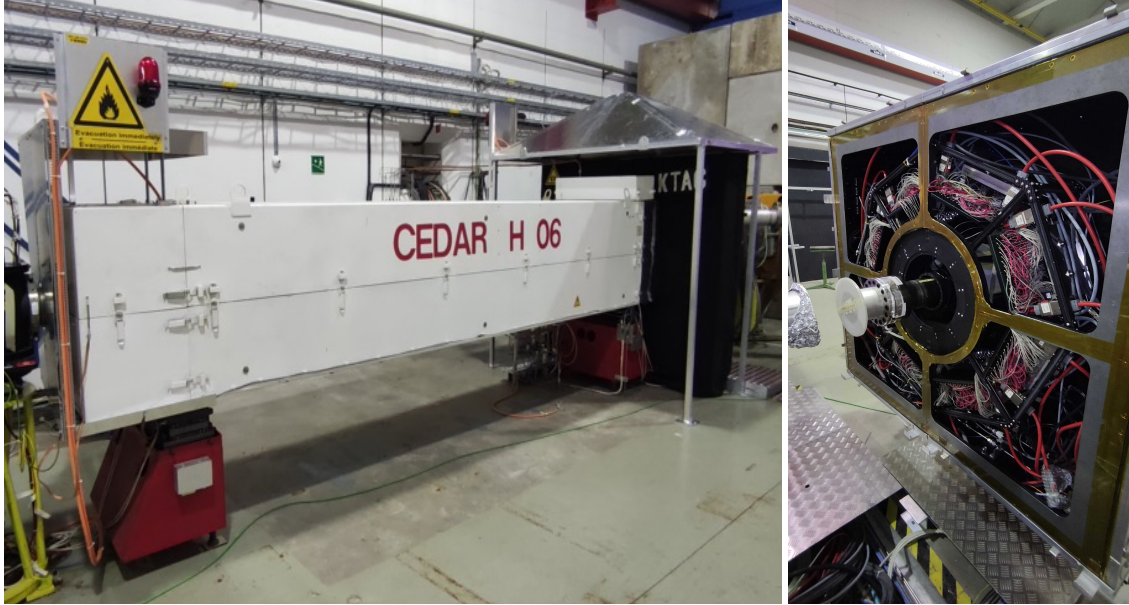
Figure 9: CEDAR-H (left panel) and KTAG photon-detection system (right panel) during installation in the experimental hall. In the left panel, the downstream end of CEDAR-H is on the left, and the black enclosure of the KTAG photon-detection system is on the right. In the right panel, the upstream-side of the enclosure is removed, revealing the eight sectors within.
