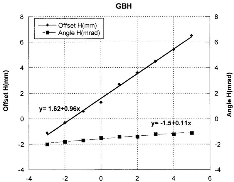
Figure 3: Variation of electron beam offset and angle with GBH and different (as compared to figure 1) currents in the other corrector coils. Both polarities of the power supply are scanned.
