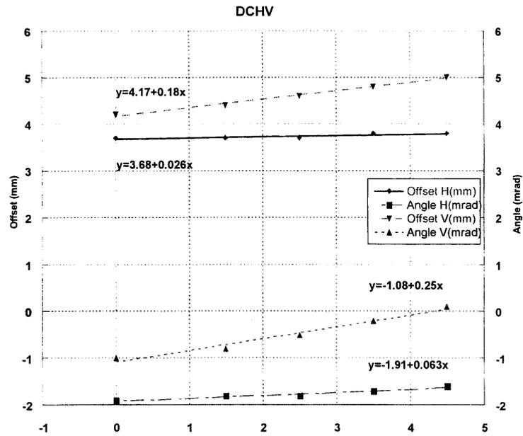
Figure 2: Variation of electron beam offset and angle with DCHV.
