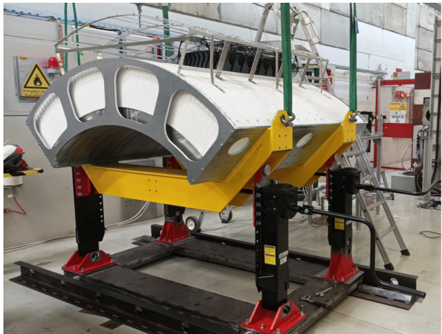
Fig. 17 The ENUBET demonstrator in the CERN T9 beamline. The white layer between the inner part of the detector and the SiPM electronics is the borated polyethylene shielding. During the test, only 20% of the detector (length: 80 cm, 18^\circ coverage in the azimuthal angle) was instrumented grouping the fibers and steering them to the SiPM boards located on top of the black plastic guides above the shielding. A test with an increase of the readout fraction by a factor 3 has been performed in August 2023.
