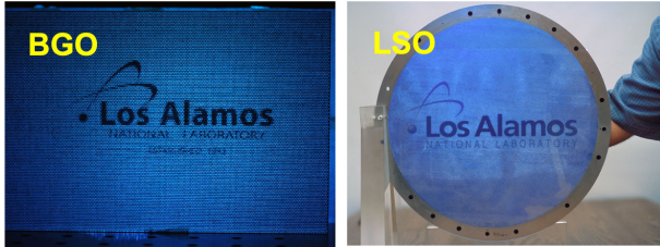
Fig. 9. Segmented BGO and LSO [98] scintillators. Both have 1 \times 1 \times 40 mm scintillator pixels and are separated by a metal septum.
