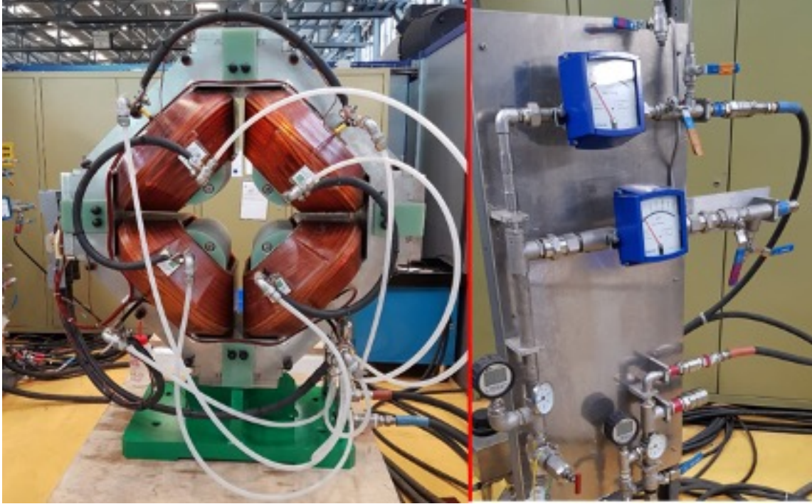
Figure 5. Water Pressure Test.
