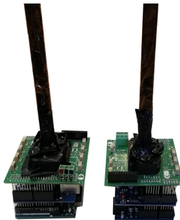
Figure 2. Scanning fiber scintillator detector.
