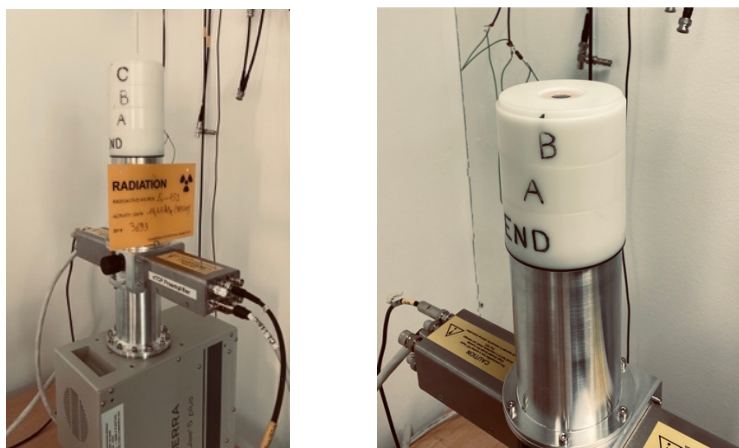
Figure 4. HPGe at n\_TOF at CERN
