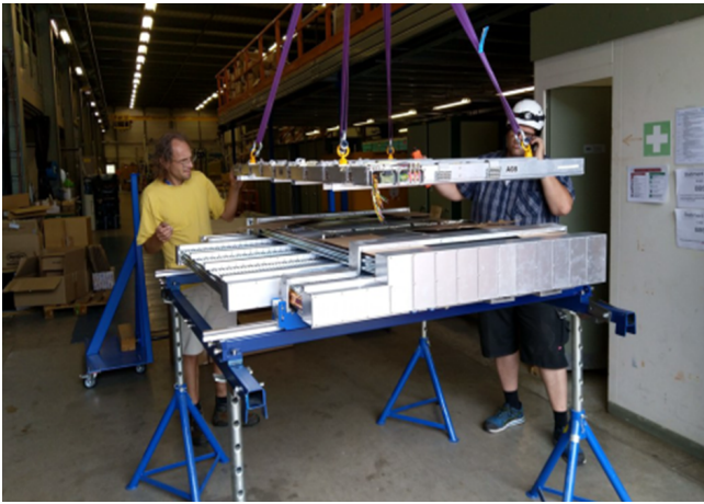
Fig. 4. Photograph of the sMDT and RPC detectors integration process.
