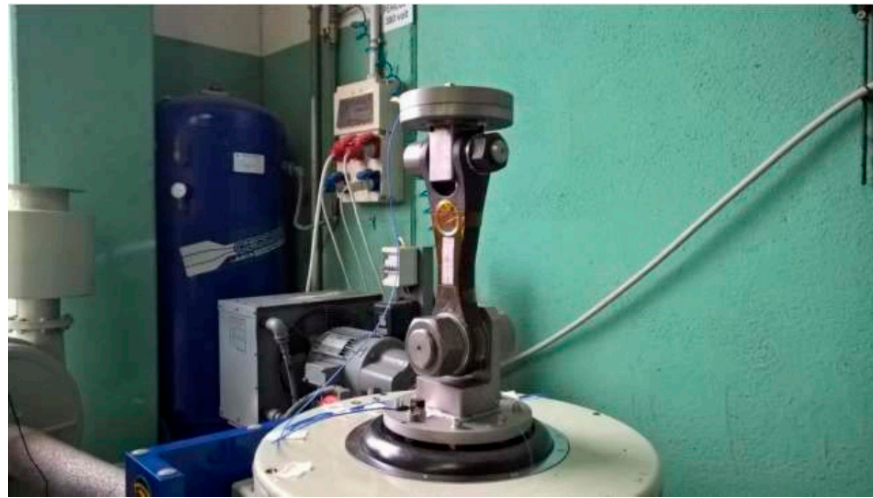
Figure 20. Experimental test setup for the vibration tests.
