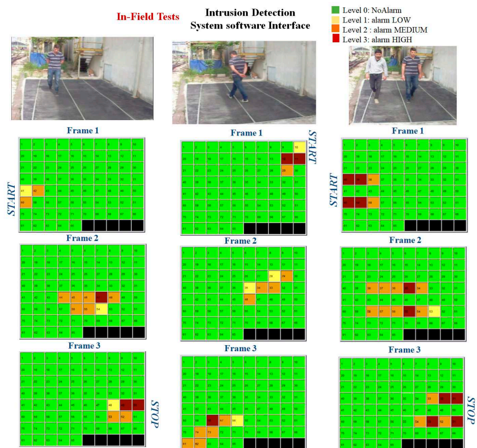
Figure 22. In-field test of the intrusion detection system. Reproduced with permission from ref. [161] (the figure is released under a Copyright Clearance Center's RightsLink® service).
