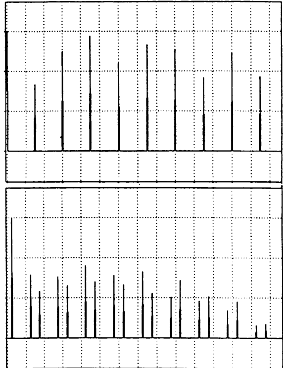
Fig.3 - Simulated results with optimum switching pattern ( N_s=66, M=0.25, 200 Hz/div, 20 dB/div) top: Harmonic spectrum of converter output voltage bottom: Harmonic spectrum of supply current
