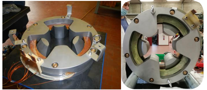
Fig. 12. The round coil superferric magnet based on MgB 2 coil: single module (left) and double module tested in 2022 (right).
