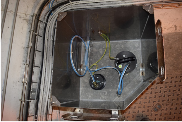
Figure 2: Vibrometers placed inside the Point 5 seismic station: strong motion sensor (left) and broadband sensor (right).
