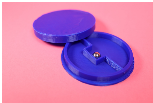
Fig. 4. Picture of the inner structure of a 3D-printable mystery box including a steel ball.
