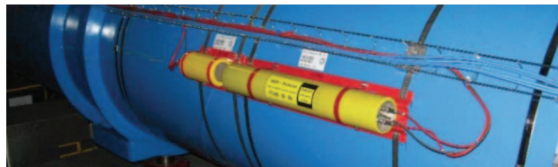
Figure 2: IC and LIC pair installed on a LHC dipole magnet.
