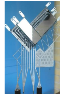
Fig. 15. Prototype 3D printed Titanium cooling plate and support structure, as part of the Upgrade I R&D phase.
