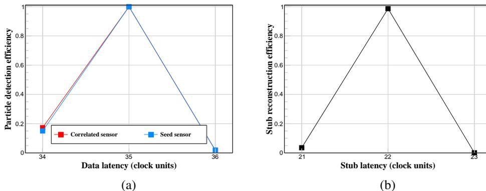
**Figure 11.** (a) Particle detection efficiency for each sensor at different values of the data latency. (b) Stub reconstruction efficiency at different values of the stub latency. The latencies are measured in units of 40 MHz clock cycles. Results are shown for the unirradiated module.
