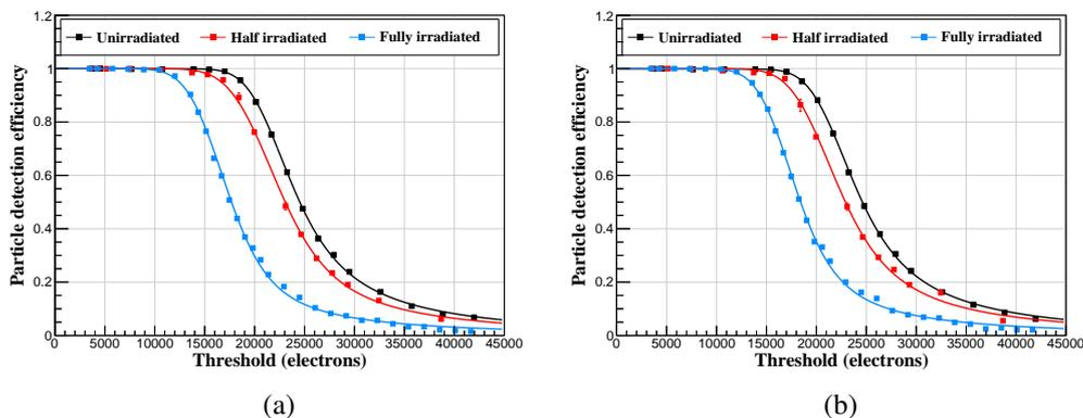
**Figure 28.** Particle detection efficiency as a function of the threshold, using selected tracks pointing within  $\pm 5 \mu\text{m}$  around the strip center, for the (a) seed sensor and (b) correlated sensor. Superimposed on each scan is the best fit performed with the integral of a Landau function convolved with a Gaussian function.
