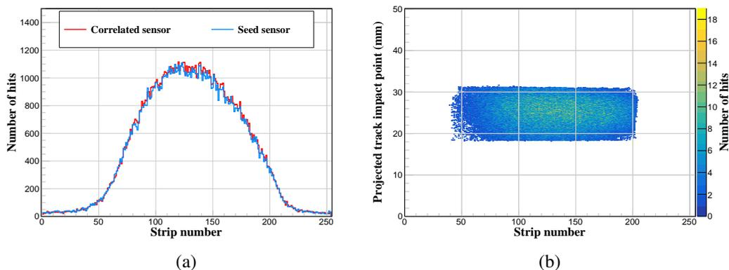
**Figure 7.** (a) Distribution of hits for the seed and correlated sensors of the unirradiated mini-module. (b) 2D hit map where the  $x$ -axis represents the strip number and the  $y$ -axis the projected track impact point along the strip direction.
