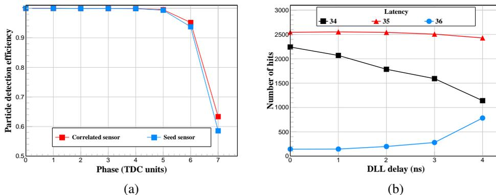
**Figure 12.** (a) Particle detection efficiency as a function of the TDC phase, in units of 3.125 ns for the seed and correlated sensors of the unirradiated mini-module. (b) Number of hits as a function of the DLL delay for three different latencies.
