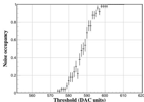
**Figure 8.** Single channel S-curve for the unirradiated mini-module.
