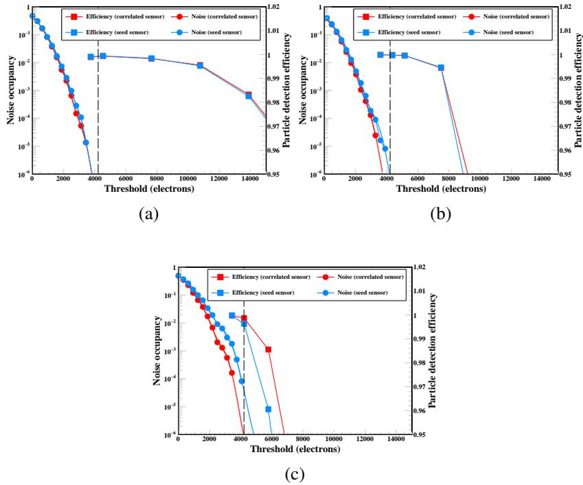
**Figure 14.** Particle detection efficiency and noise occupancy as a function of  $V_{\text{TH}}$  for the unirradiated (a), half irradiated (b), and fully irradiated (c) mini-module. The dashed lines correspond to the optimal threshold.
