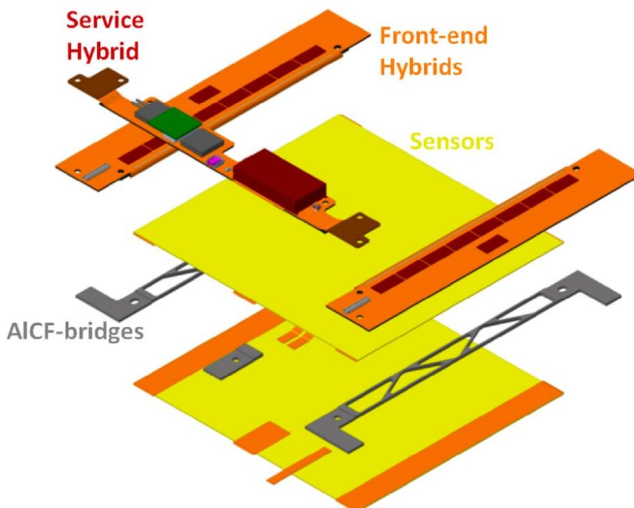
**Figure 2.** Exploded view of a 2S module. The seed and correlated sensors, in yellow, are separated by two aluminum carbon fiber bridges. The two front-end hybrids, in orange, are mounted on the two sides of the sensors. The service hybrid, in red, with two DC-DC converters inside an electro-magnetic shielding box and the optical link to the DAQ, is mounted between the two front-end hybrids.
