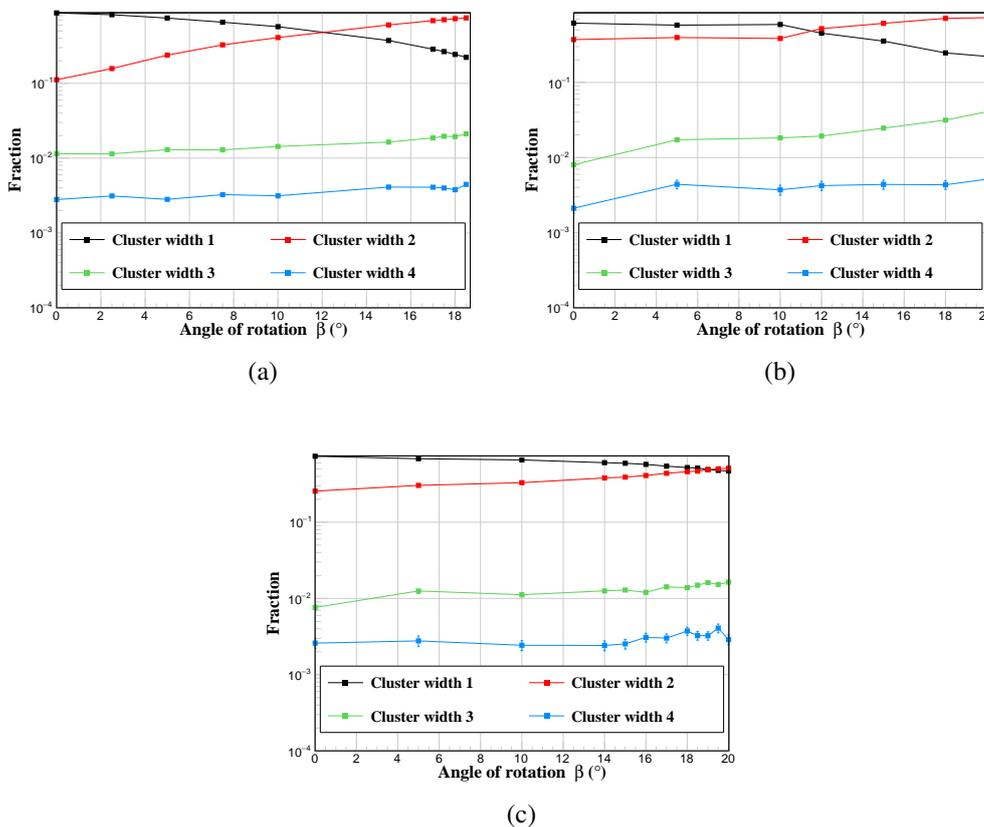
**Figure 22.** Fraction of clusters with different widths shown as a function of the incident angle. Results are shown for the correlated sensor of the (a) unirradiated, (b) half irradiated and (c) fully irradiated mini-module.
