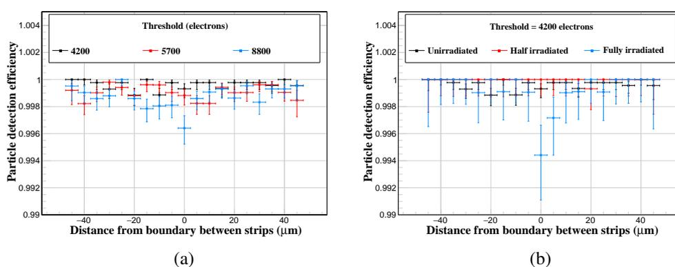
**Figure 18.** Particle detection efficiency as a function of the track location with respect to the center between adjacent strips for different thresholds of the unirradiated mini-module (a) and for different irradiation fluences (b).
