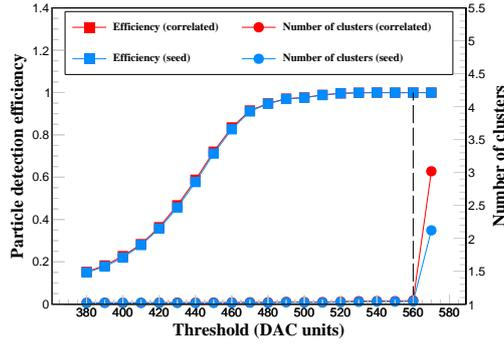
**Figure 13.** Particle detection efficiency and number of clusters detected per event as a function of  $V_{\text{TH}}$ , for the unirradiated mini-module. The dashed line corresponds to the optimal threshold.
