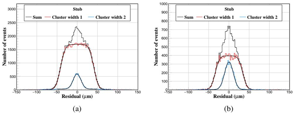
**Figure 25.** Stub residual distributions for the unirradiated (a) and fully irradiated (b) mini-module. The cluster of width one distribution was fitted using a constant linear function convolved with a Gaussian function. The cluster of width two distribution was fitted using a Gaussian function with an offset.
