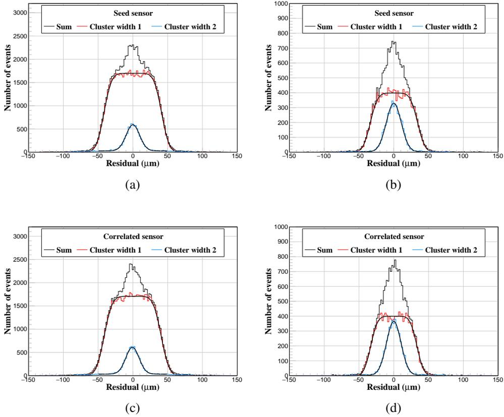
**Figure 24.** Residual distributions for clusters of width one and two for the unirradiated (a), fully irradiated (b) seed and unirradiated (c), fully irradiated (d) correlated mini-module sensors. The cluster of width one distribution was fitted using a constant linear function convolved with a Gaussian function. The cluster of width two distribution was fitted using a Gaussian function with an offset.
