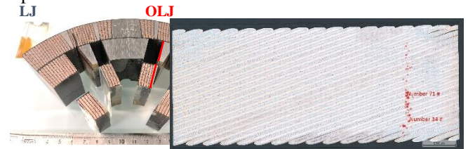
Fig. 9. MQXFA08 quadrupole magnet coil AUP 213: OLJ side inspection. The red marks on the prepared longitudinal cross-section represent all transverse crack-events (approx. 105) within a narrow field (2 mm wide) at the resin-Cu wedge interface.
