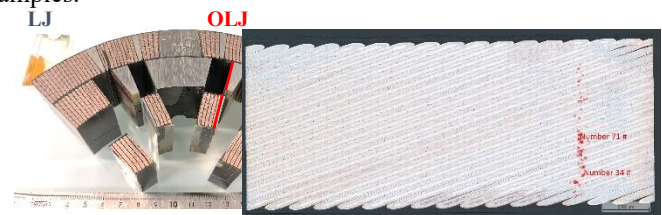
Fig. 9. MQXFA08 quadrupole magnet coil AUP 213: OLJ side inspection. The red marks on the prepared longitudinal cross-section represent all transverse crack-events (approximately 105) within a narrow field (2 mm wide) at the resin-Cu wedge interface.
