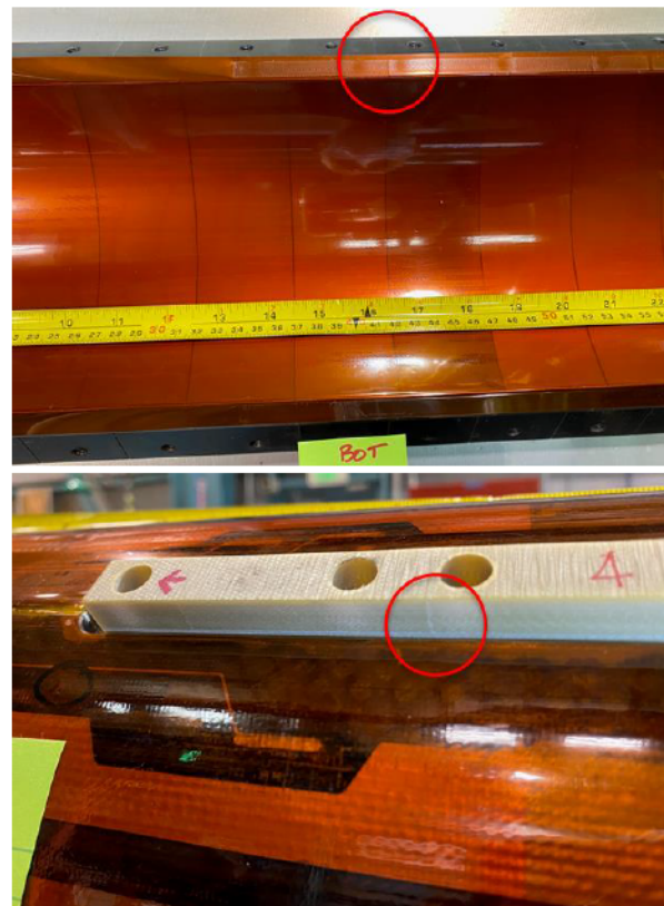
Fig. 7. Red circles: high pressure “imprints” of collar lamination on the polyimide insulation between the collars and pole keys (top) and on the pole keys of Q3 (bottom).
