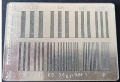
Figure 4. Line pair mask type 17 made of 0.02 mm thick lead used as an imaging target. For this particular mask, 0.5 LP/mm means that one black and one white line within 2 mm will be projected on the image sensor.
