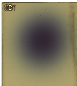
Figure 1: Gafchromic EBT3 film irradiated at CLEAR.
