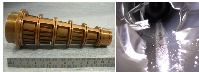
Figure 1: (a) GlidCop® core, (b) damaged Ni coating [2].
