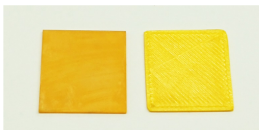
Figure 8. Left: ZnSe:Al single crystal. Right: 3D printed scintillator with ZnSe:Al granules.
