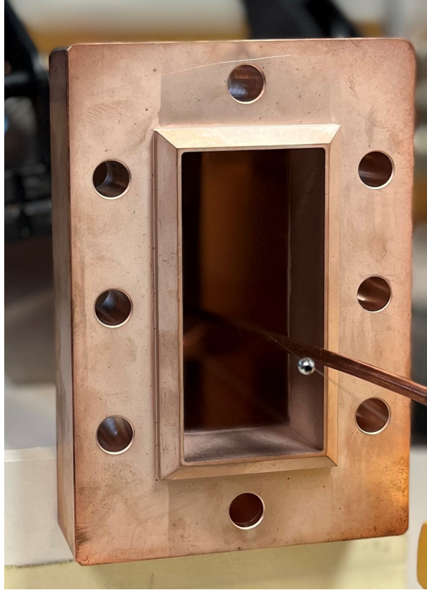
Figure 4.3: Zoom on the positioning of the antenna inside the rectangular pipe of the pill-box like cavity involved in the bead-pull measurements.
