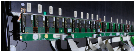
Figure 2: Left panel: DUAL SAMPa front-end electronics board for the MCH. Right panel: new MCH readout chain for Run 3.
