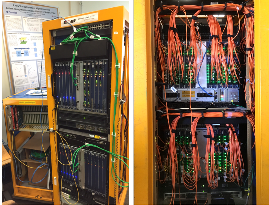
Figure 9: Demonstrator hardware rack. The Data Source boards are in the lower ATCA shelf and the PRBs are in the upper shelf. The rear view of the rack (right) shows 120 QSFPP+ optical cables connecting the two shelves.
