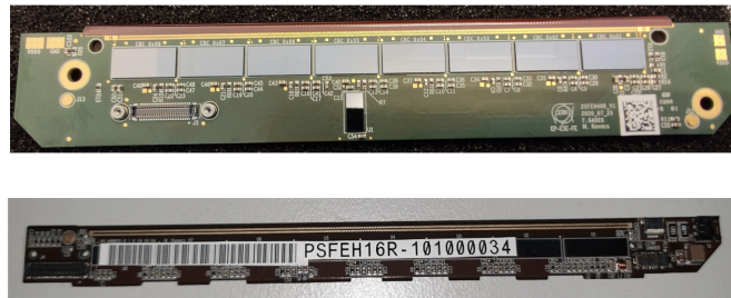
Figure 2. Top view of the 2S front-end hybrid (top) and of the PS front-end hybrid (bottom).
