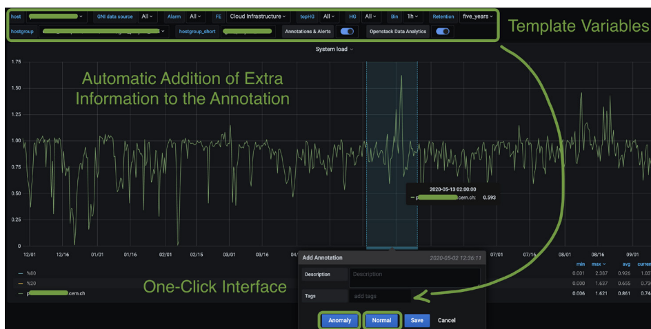
Figure 6. Modification introduced in the Grafana annotation interface: “Normal” and “Anomaly” buttons are available in the annotation input form, and the dashboard’s template-variables are automatically appended as annotation’s tags.
