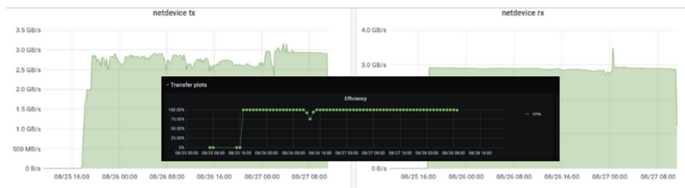
Figure 6: Large test from EOS to CTA (675 TB) with Rucio. CTA reading and writing throughput between the tape buffer and tape (behind) and FTS efficiency (in front)
