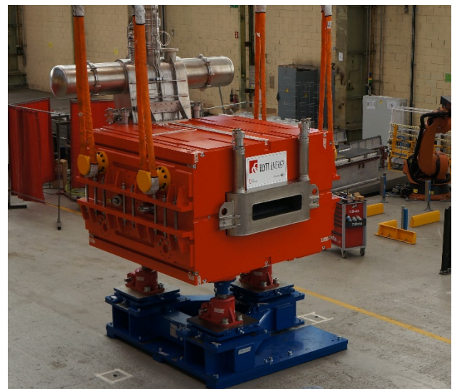
Figure 5: First of Series dipole ready at Elytt to be packed for shipment.
