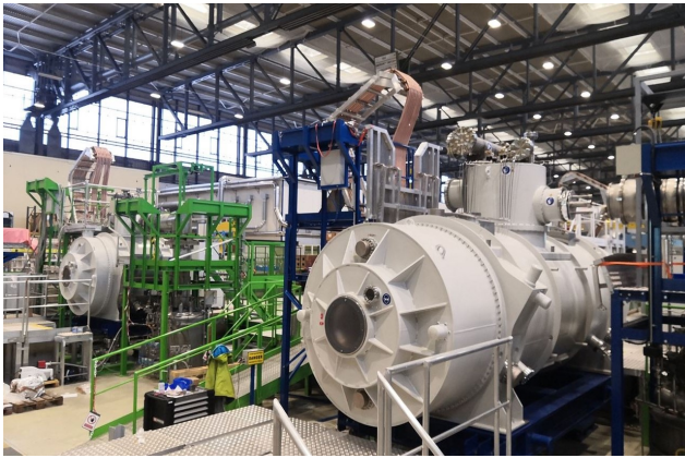
Figure 3: Long (in the front) and short multiplet mounted on test benches at CERN layout of FAIR.
