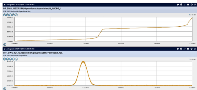
Figure 1: The top plot shows position data for both in and out scan. On the bottom plot beam profile data is displayed.
