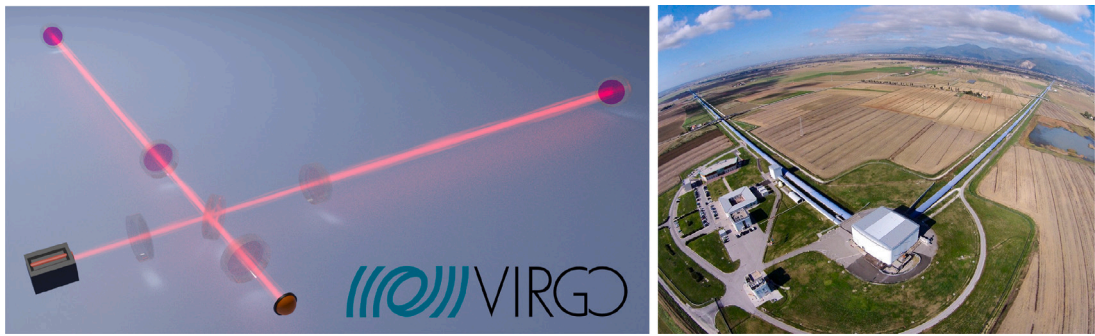
Fig. 20. Schematic diagram of the second generation interferometric gravitational wave detector. For simplicity, only the main optic elements are depicted. Left: laser source and detection are schematically depicted as black box and orange semi-circle. Right: Virgo aerial view. The two 3-km arms of the interferometer meet the central building where the laser is generated, and five mirrors, including the beam-splitter mirror, are hosted. Optical benches used to acquire the interference pattern are also hosted in this building. On the left part, the other buildings host EGO offices. Credits: the Virgo Collaboration/N. Baldocchi. (For interpretation of the references to color in this figure legend, the reader is referred to the web version of this article.)
