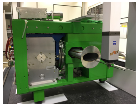
Figure 7: Photo of the steel shielding-covered dump on a CMM machine.
