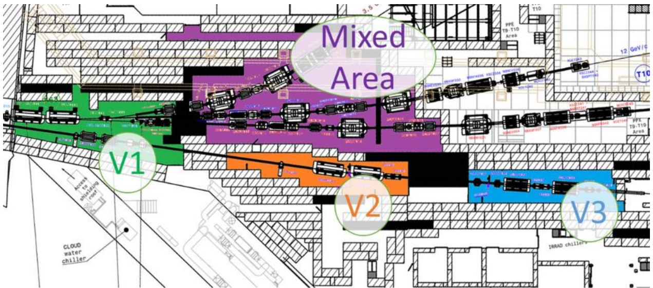
Fig. 5-12: Location of the primary zone bunkers (V1, V2, and V3) and the mixed area.
