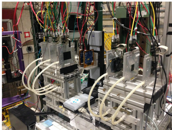
Figure 4. Test beam setup at the North Area of CERN SPS. Here two sensors are placed between the telescope planes.
