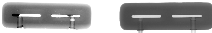
Fig. 21. X-ray of solder joints attaching the fluidic connector to the microchannel cooler. The left image demonstrates an unsuccessful soldering in which solder has crept into the slit regions. Voids connect to the slits are also visible. The right image demonstrates a successful soldering, with no voids or solder excess.
