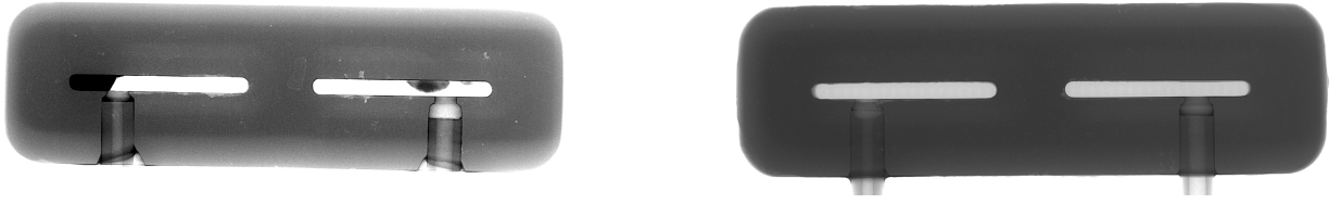
Figure 20: X-ray of solder joints attaching the fluidic connector to the microchannel cooler. The left image demonstrates an unsuccessful soldering in which solder has crept into the slit regions. Voids connect to the slits are also visible. The right image demonstrates a successful soldering, with no voids or solder excess.
