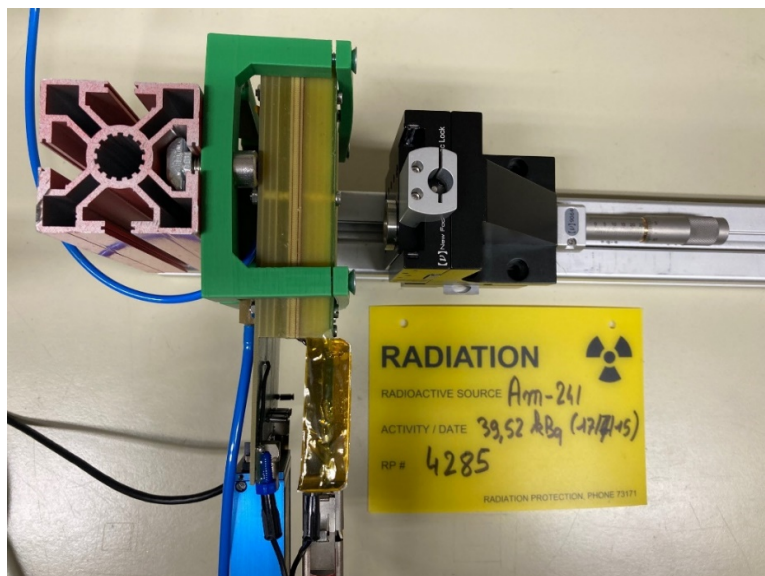
Figure 3. The ^{241}\text{Am} source is placed on a holder such that its distance from the GEMPix can be adjusted by a micrometer screw.
