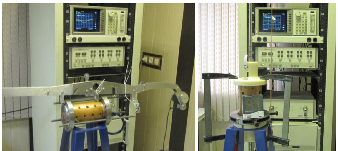
Figure 13. Bead-pull measurement and tuning setup.
