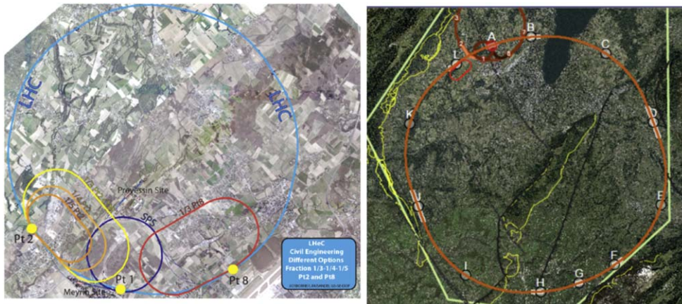
Figure 7. Possible locations of the ERL racetrack electron accelerator for the LHeC (left) and the FCC-he (right). The LHeC is shown to be tangential to Point 2 and Point 8. For Point 2 three sizes are drawn corresponding to a fraction of the LHC circumference of 1/3 (outer, default with E_e = 60 GeV), 1/4 (the size of the SPS, E_e \simeq 55 GeV) and 1/5 (most inner track, E_e \simeq 50 GeV). Civil engineering chose point L as the position of the ERL at FCC, with two GPDs located at A and G.
